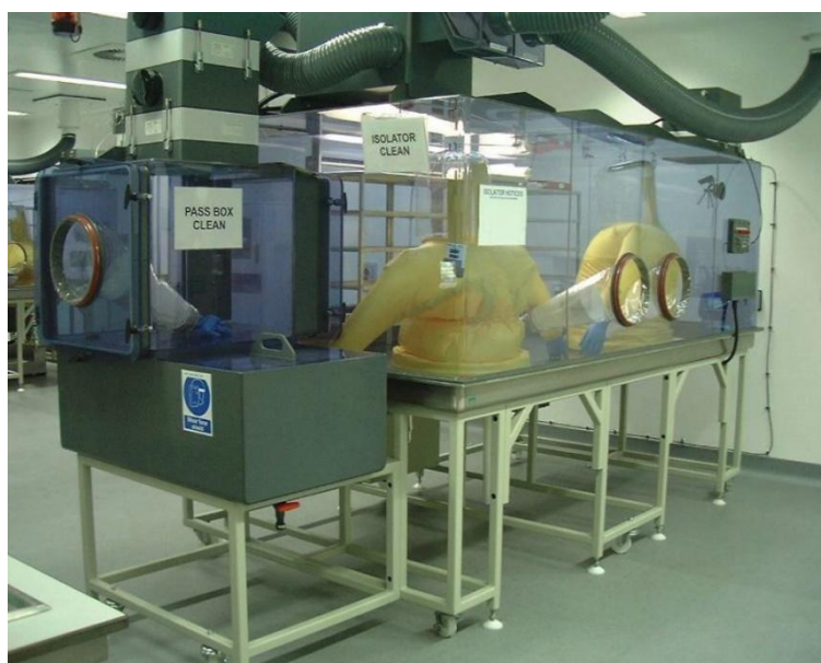
Figure 16. A solid frame isolator used in a BSL-4.
