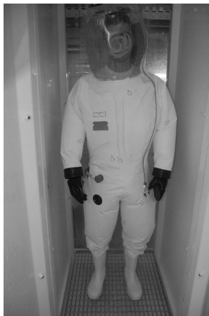
Figure 17. A Honeywell BSL-4 positive pressure suit in a decontamination shower mock up.
